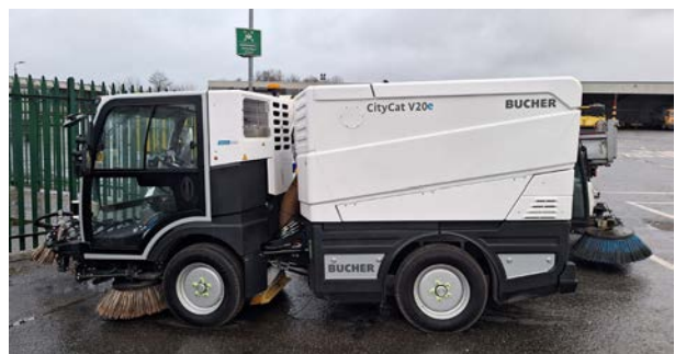
Figure 27: EV Powered Fuel sweeper on fleet
