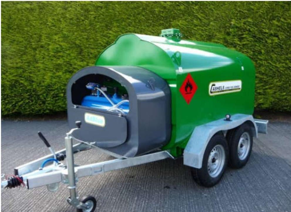
*Figure 3.1 - Typical mobile fuel bowser (Source: Clarke Machinery Group)*
